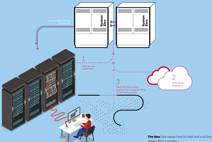
The situation Millions of gigabytes of data are processed and stored in computer centres, with around 40% of energy consumption going on cooling alone. This produces an enormous amount of waste heat (approximately 548 MWh/year for 100 kW of cooling). This is energy that was unused in the past.
